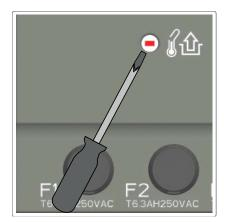
figure 28 - Resetting the safety thermostat
