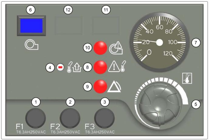
figure 2 - Thermostat module
