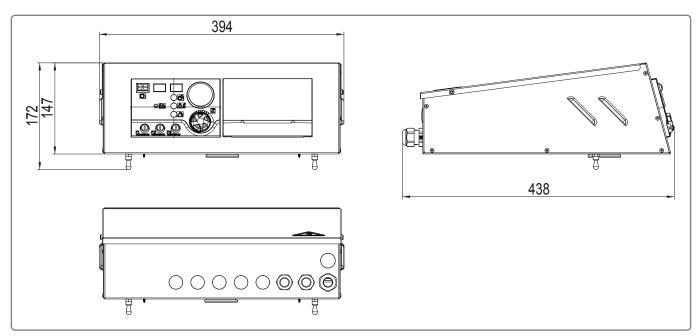
figure 1 - Dimensions (in mm)
