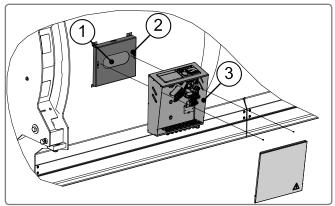
figure 6 - Fitting the control panel
