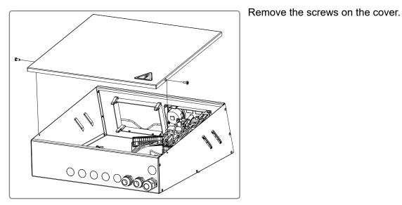
figure 4 - Opening the control panel
