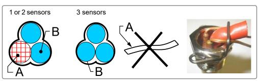
figure 9 - Installation of sensors
