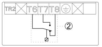
figure 23 - Connection of external control
