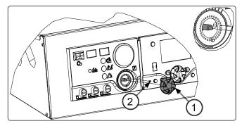
figure 26 - Positioning the thumbwheel's stopping pin
