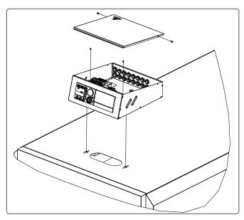
figure 5 - Fitting the control panel
