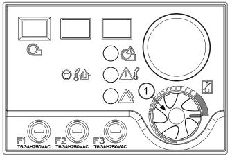
figure 25 - Thumbwheel in maximum position
