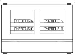
figure 24 - Time and pulse meter
